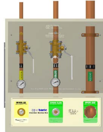
Shown above model HCBU3OHW2A6VT Two valve+ One vent box with gauges 3/4” oxygen, 1/2” medical air, 1 1/2 vent
