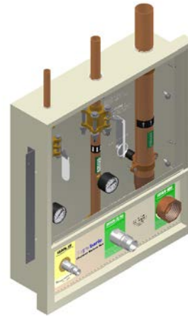
Shown above model HCBU3OHW2A6VT Two valve+ One vent box with gauges 3/4” Oxygen valve & high flow oxygen (without check), 1/2” medical air, 1 1/2 oxygen vent
