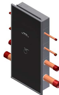
Shown above EVU4R2AB2NB3OB4VS 4 valve box with gauges ½” Medical Air, ½” N 2 O, ¾” Oxygen, 1” Medical Vacuum
